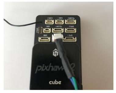
2. Wiring scheme of Molex 4 pin connector to pixhawk "TELEM1" 8 pin connector. **WARNING: Do not plug in the +5V wire**. Please plug in only 3 wires (Tx, Rx, GND) on the 4 pin MOLEX connector
