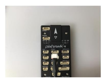
Wiring scheme of Molex 4 pin connector to pixhawk "TELEM1" 8 pin connector.
