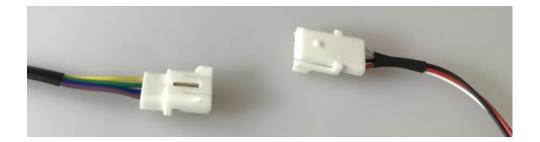
3. Power plug the Pixhawk 4 via USB port from PC, turn on the camera. (you can plug in the GPS module for testing if you want) **WARNING: Do not plug in the +5V wire**. Please plug in only 3 wires (Tx, Rx, GND) on the 4 pin MOLEX connector
